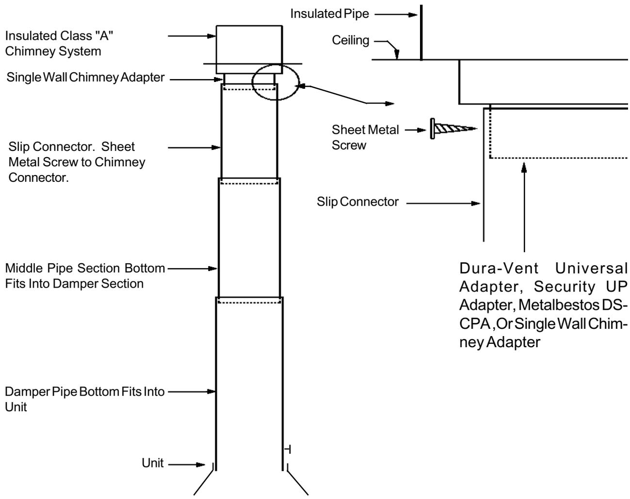
The above illustration represents the installation procedure for dripless pipe installation. This installation method of installing the connector pipe with the male end down allows for any moisture to remain on the inside of the connector pipe.
