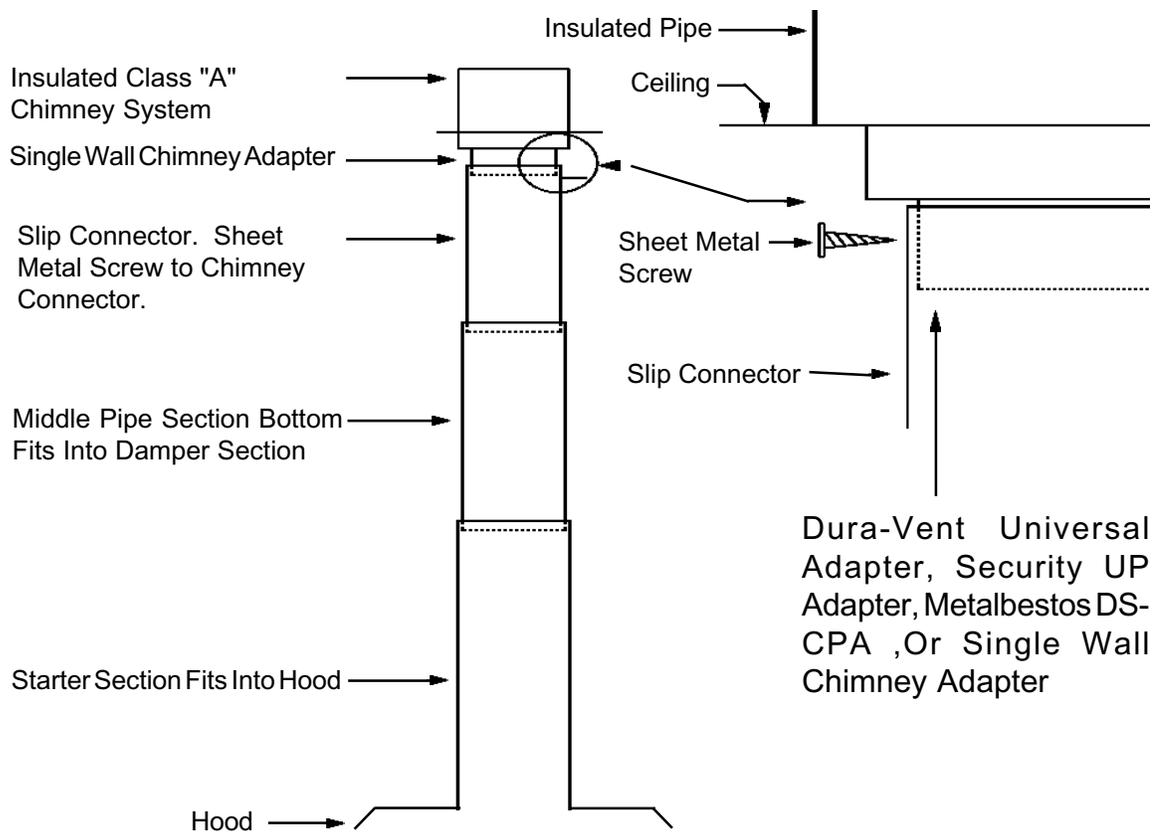
The above illustration represents the installation procedure for dripless pipe installation. This installation method of installing the connector pipe with the male end down allows for any moisture to remain on the inside of the connector pipe.
